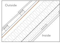
DAFA RooFoil 230 MH used as roof decking with ventilation between insulation and roof decking.
