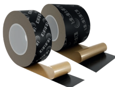
DAFA UV tape is a UV-resistant, single-sided polyethylene tape which is ideal for sealing and affixing roof underlays and wind barriers outdoors.
