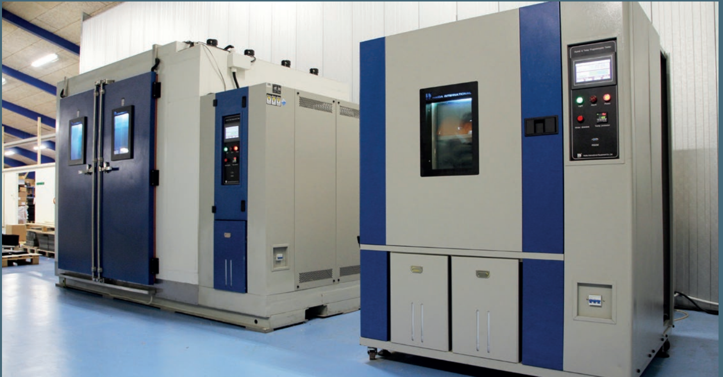
DAFA's climate testing chambers at Holmstrupgaardvej in Brabrand.
