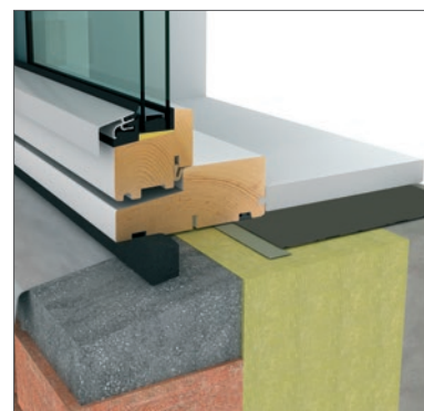
DAFA Duo Foil lining foil in window structure.
