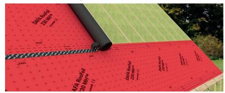
DAFA RooFoil 230 MH Plus is installed with an overlap of minimum 150 mm. Self-adhesive borders in both sides ensure optimal adhesion.
