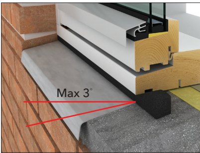
9A. We recommend max. 3° sill pitch.
