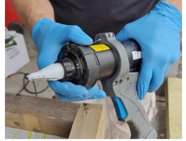
Screw the entire top (with the 2 caulk nozzles) into place. Must be thoroughly tightened.
