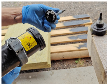
When the bag is empty, unscrew the top and remove the long caulk nozzle.
