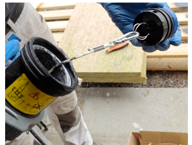
The bottom plug is attached with a wire or chain. Reinsert this before placing a new bag in the tube.
