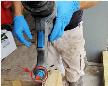
The compressed air valve should be fully open when spraying. Close slightly if necessary as needed. Adjust to a suitable level.
