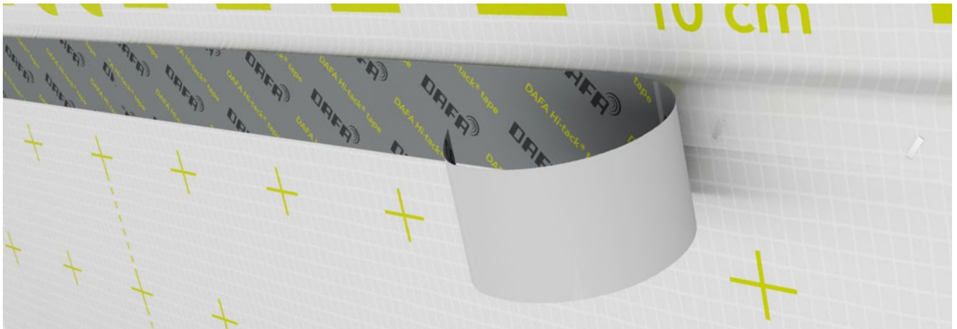
DAFA ExFoil is installed with an overlap of min. 100 mm and can be taped e.g. with DAFA Hi-tack® vapor barrier tape. The new DAFA Zero Waste tape can also be used.
