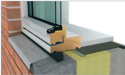
External joints using illmod 600 sealing tape. Interior airtightness with DAFA joint foils.
