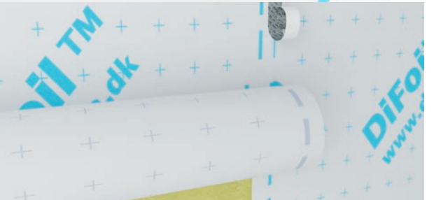
DAFA DiFoil consists of polyethylene (PE) material with a moisture-absorbing polypropylene (PP) fleece layer. The material can withstand direct sunlight for up to three months, and must not be exposed to direct contact with wood preservative with added solvents.
